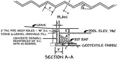
2. Sloped seawall: The top portion of the wall, from elevation 739 to its highest elevation, is angled away from the lake at a 30-degree angle (see illustration).
